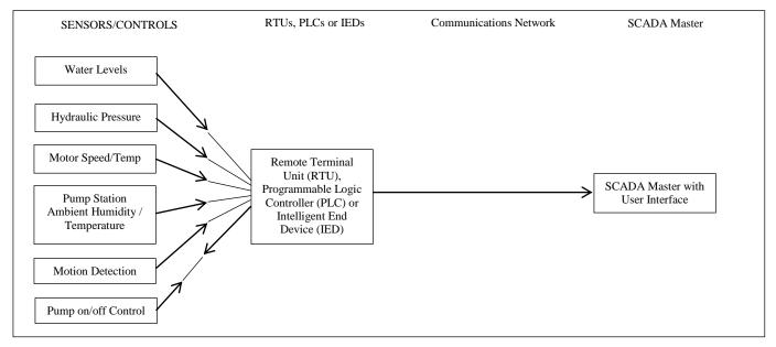
Figure 1. SCADA Components
