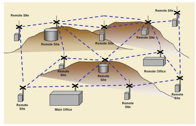
Figure 2. Typical SCADA Communication Network Configuration
